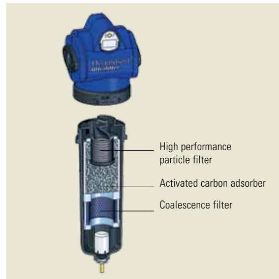
Cross-section of an Ultra-Filter with DF-T element
