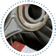
**Needle bearing** in both connecting rod eyes
