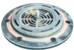
stage valve of an air-cooled compressor after 2,500 hours
