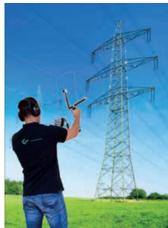
Checking high-voltage overhead lines for corona discharge
